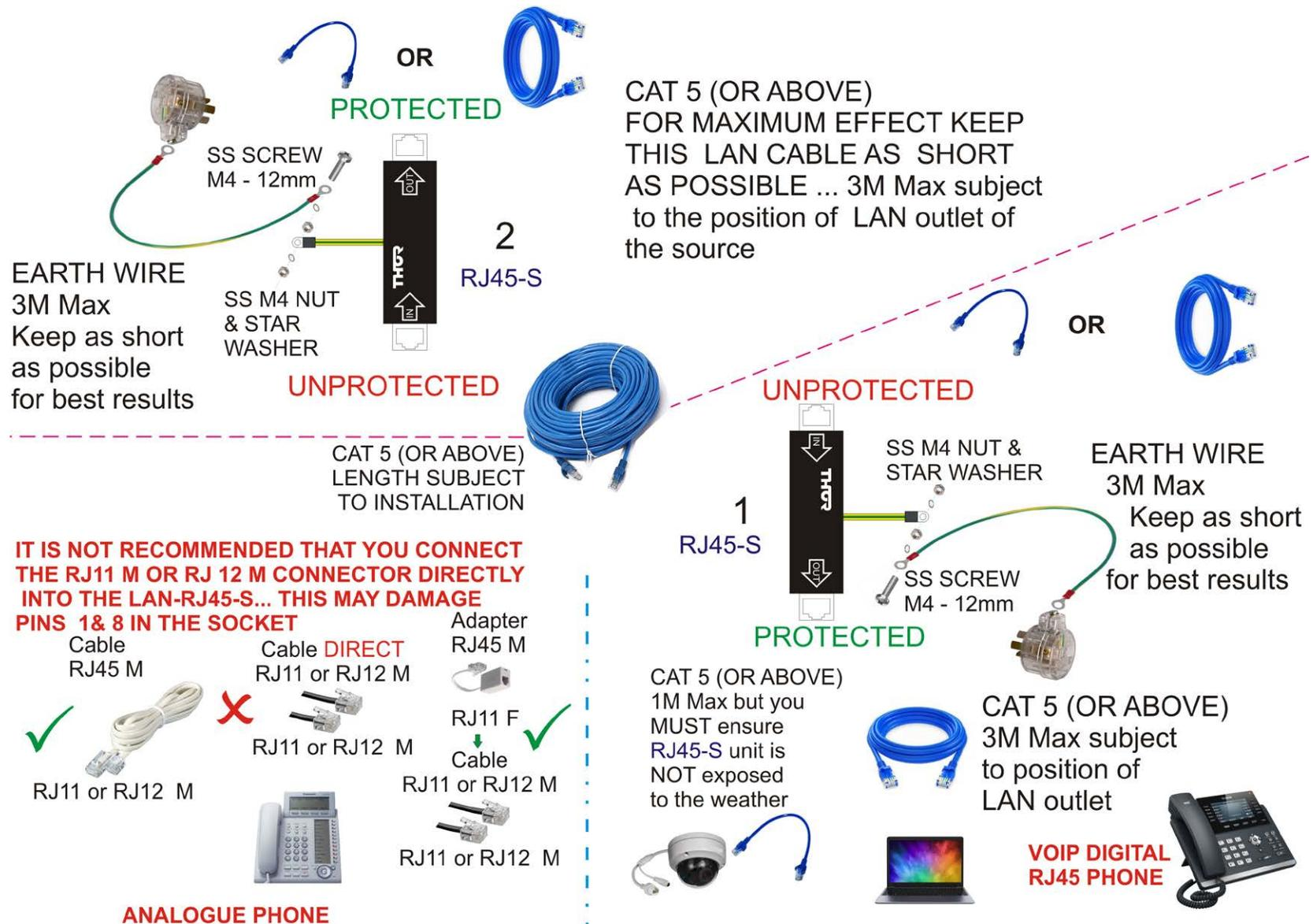
For product only protection follow wiring guide as per '1' for protection at both ends follow wiring guide for both '1 & 2'
